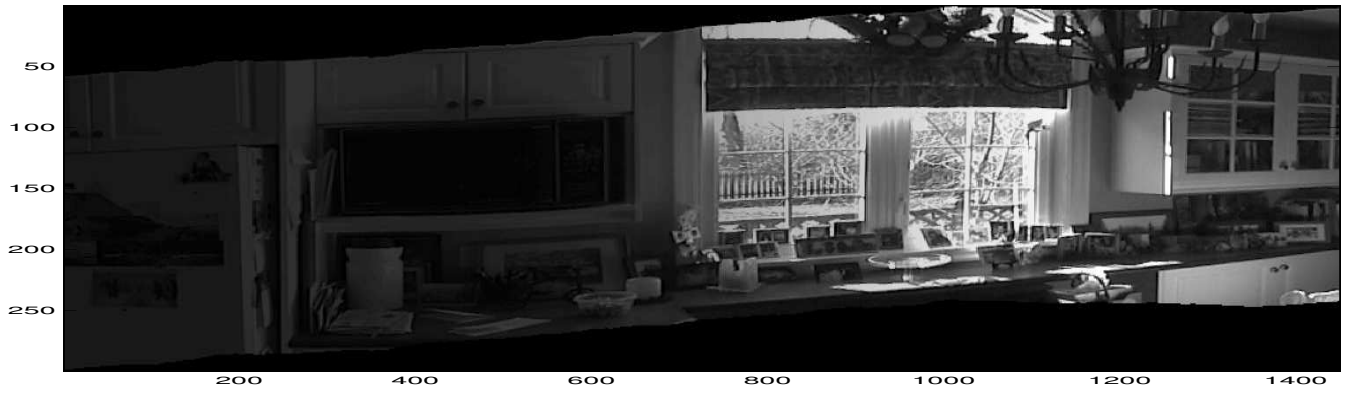
Fig. 9: Spatially and tonally aligned strip mosaic for a high dynamic range kitchen sequence. This greyscale image displays the square root of the photoquantity panorama
