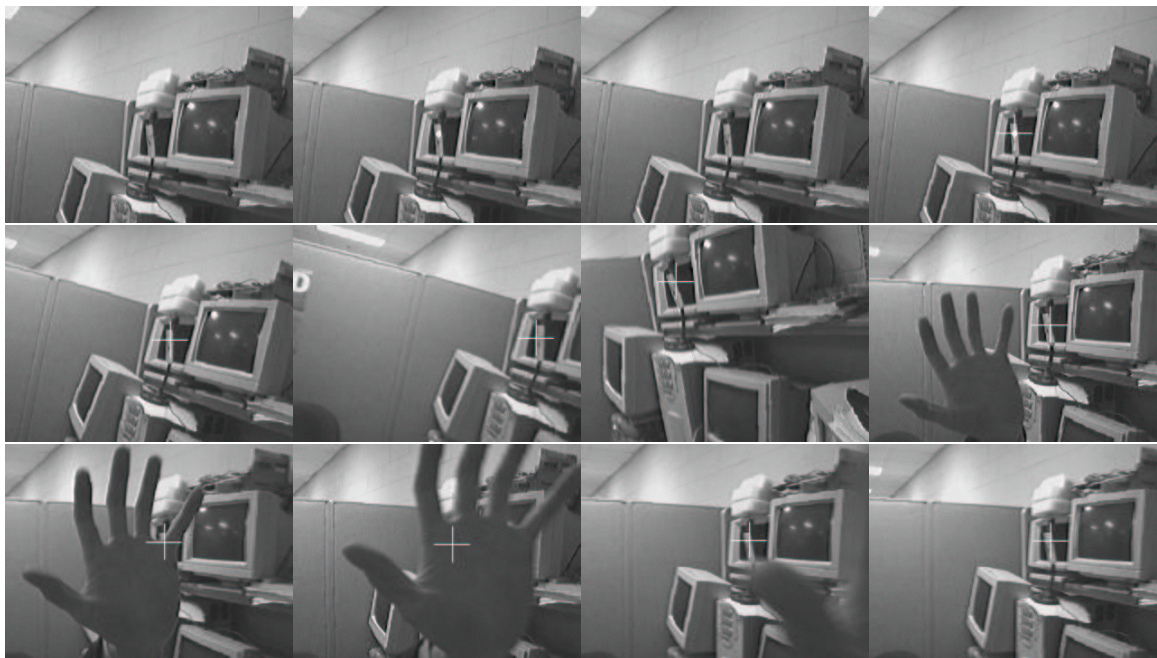
Figure 9: MRBDL in action: the first sequence of four images shows VIS locating the beacon attached to the monitor. Notice that the beacon toggles on and off in subsequent images. The next three images show the OTS correctly positioning the crosshairs on the disengaged beacon's location in spite of significant head movement. The final five images illustrate the gyro-assisted OTS's ability to track devices even in the presence of independently moving objects.
