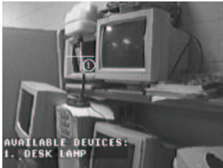
Figure 3: The user interface: through they EyeTap, the user sees one Bluetooth-enabled desk lamp in range, which is being tracked.
