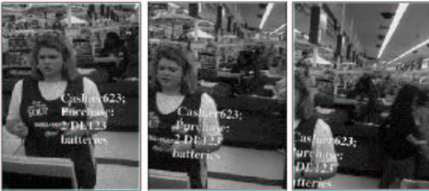
Figure 1: An annotation overlay fixed to the scene using projection motion tracking. By applying the best fit projective coordinate transformation found between frames of video to the overlaid text, the annotation appears as a planer object that is part of the scene. This makes for us to maintain our immersion in the real environment as well as making it easier to interpret the text.
