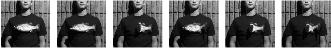
Figure 1: The wearable physical avatar in the form of a talking fish. The mouth of the fish moves in synch with the voice as it talks, whereas the tail follows a Poisson distributed random variable, and the head moves as well (3 degrees of mechanical movement).
